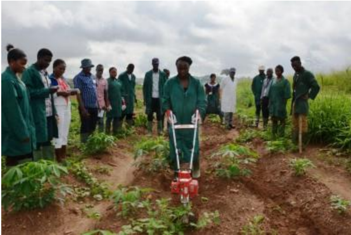
Figure 3 Mechanical Cassava Weeder Developed by IITA 4
